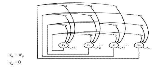
• weights: fully connected, symmetric, and zero diagonal.
